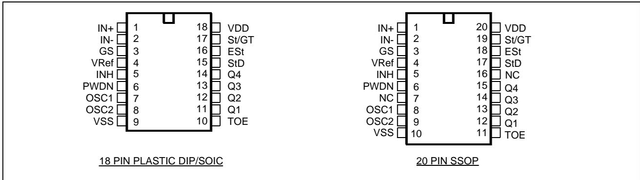
Figure 2 - Pin Connections
