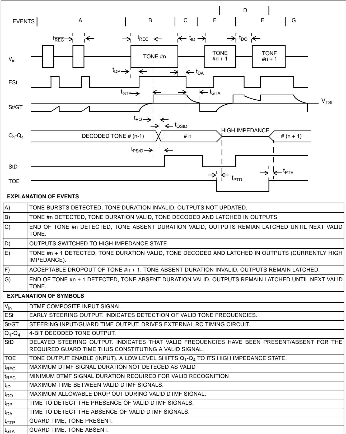
Figure 11 - Timing Diagram
