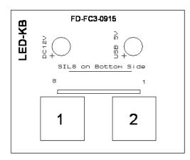
Keyboard PCB has two 12mm push buttons and two LEDs for power indication.
