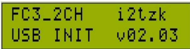
FC3 is waiting to be recognized by Windows and needed drivers are installed.
