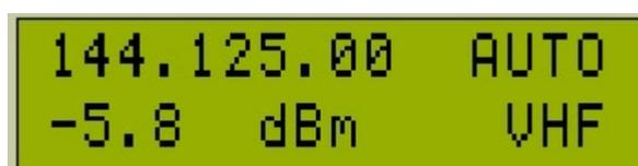
HF mode can read frequencies up to 60 MHz, VHF uses an MC12080 prescale to divide by 10 the input frequency. AUTO will automatically select, when needed, the prescale usage.
