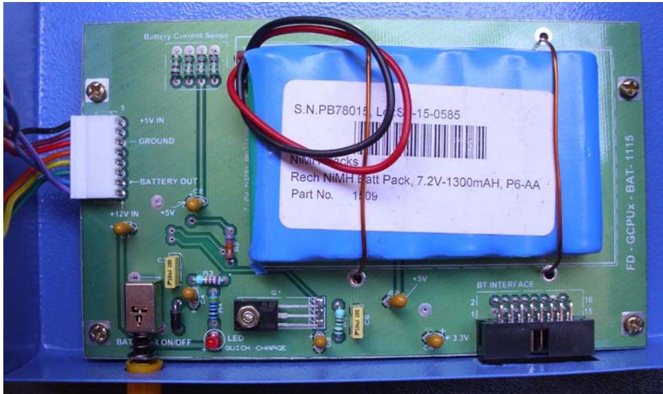
**Battery, NiMH or NiCad can be used in this board. Require a 4 Cell battery with about 1000ma capacity (more is always better!)**
