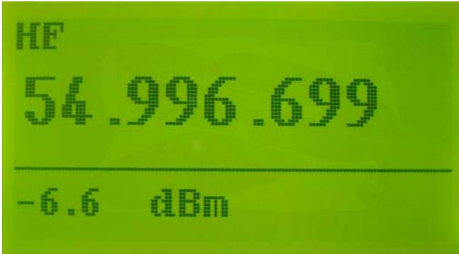
Antenna analyzer (AAZ-0914A) output connected to check frequency and signal level at 55MHZ
