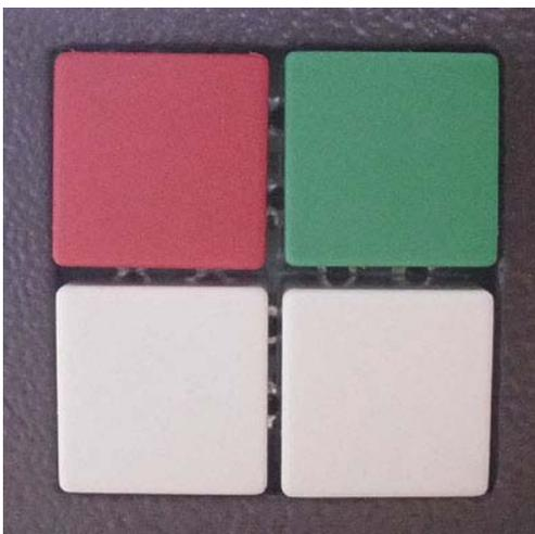
**Four Button Menu has two top buttons for selection and lower two for selection within menu.**
