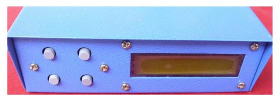
ST2 is an advanced Satellite Antenna Tracking Interface for Yaesu (Or similar) Rotor Controllers. Project uses PIC16F876A, 28PIN DIP. Firmware uses full A/D and EPROM capability of 876A and makes setup a smooth process.
