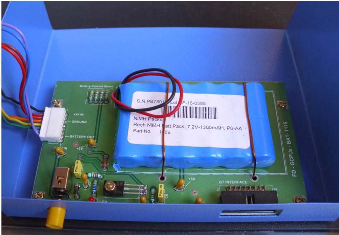
**Battery board has MAX712 battery charger, ON/OFF Switch, 5V and 3.3V regulators, charging pass transistor and space for NIMh/NiCad battery. (Battery is not included with kit or assembled due to postal regulations.**
