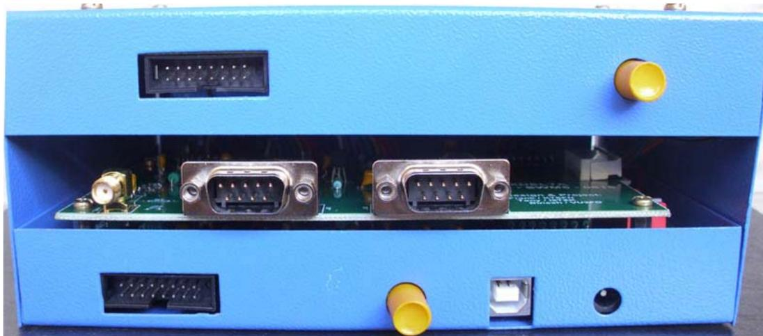
Bottom Push switch = USB / DC12V (+Battery) TOP Push Switch = Battery ON
