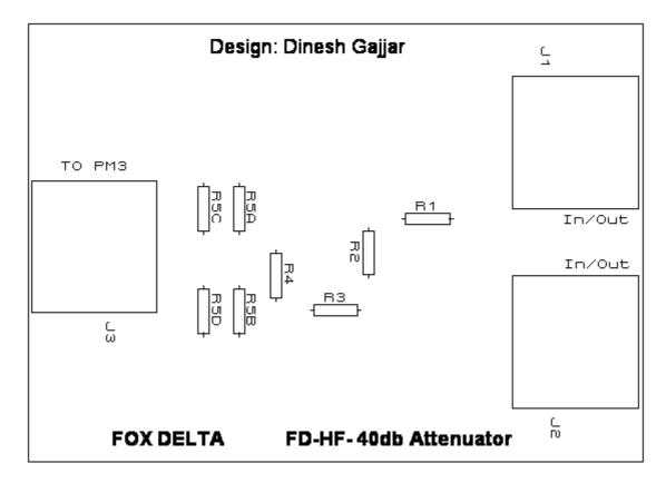
To get - 40dB a 100:1 voltage divider is made with 50 Ohm output impedance. When this output is loaded, the total load resistance would be 25 Ohm.
