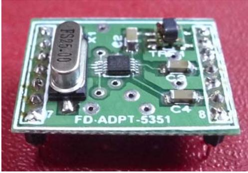
Kits are supplied with Si5351 chip Pre-soldered on a carrier board (M1) for easy assembly.
