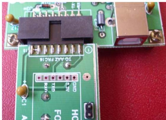
**BT module plugged into FRC16 Socket:**
