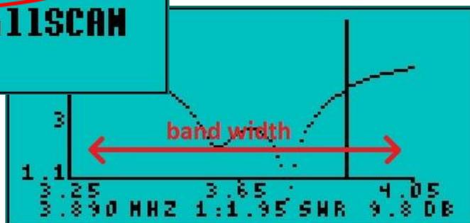
The *Frequency Center* and *Scan Width* will be used on the next scan. Until a new scan is executed the previous values are still shown on the graph display.
