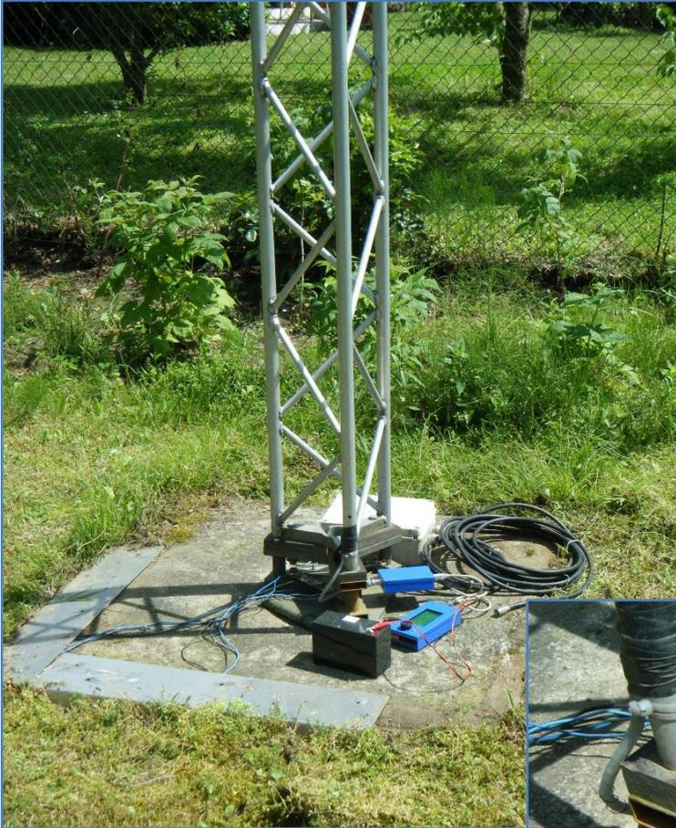
Testing an 80m 1/4 wave vertical
