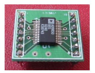
Kits are supplied with AD9850 Pre-soldered on a carrier board for easy assembly. This plug-in module is tested for full HF range before dispatch with kits.
