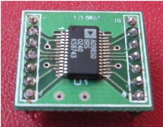
DDS: AD9850 is supplied with kits as a Pre-Soldered and fully tested for 0 to 35MHZ range.
