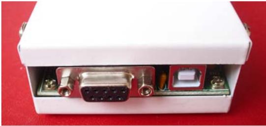
AAZ-0713A has two powering and communication options. You may connect your PC at USB or connect it to a D9M cable for Graphic CPU/DISPLAY.
