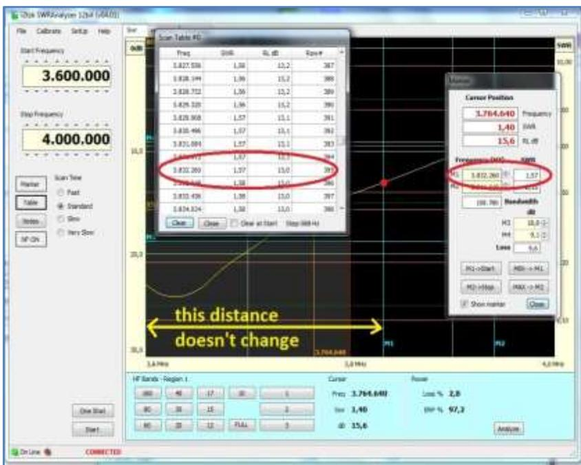
It can be seen that the values and the Scan Table & Marker windows reflect the measured values associated at the frequency, where the M1 marker intersects the graph, i.e. M1 marker is in the same position on the screen in both figures.
