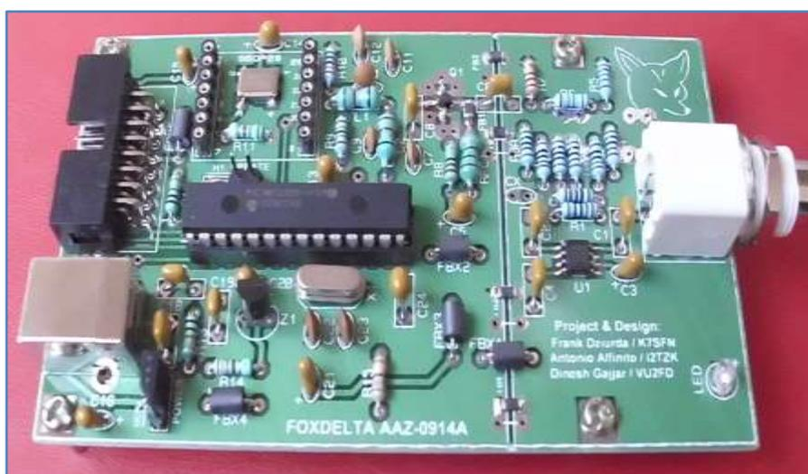
The RLB's output voltage is fed to the AD8307 (configured as detector/differential comparator), which amplifies the signal level, and converts it to a dB (decibel) level that is fed to the microcontroller.
