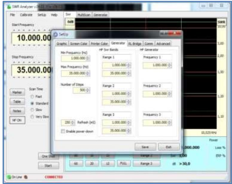
The **[SetUp] [Generator]** tab also allows you to change the min and max frequencies as the overall range the DDS is required to work over. **By default the range is 1.0 to 35 MHz** to overlap the whole of the HF bands slightly. Change the max frequency if you want to explore the 6m band too.
