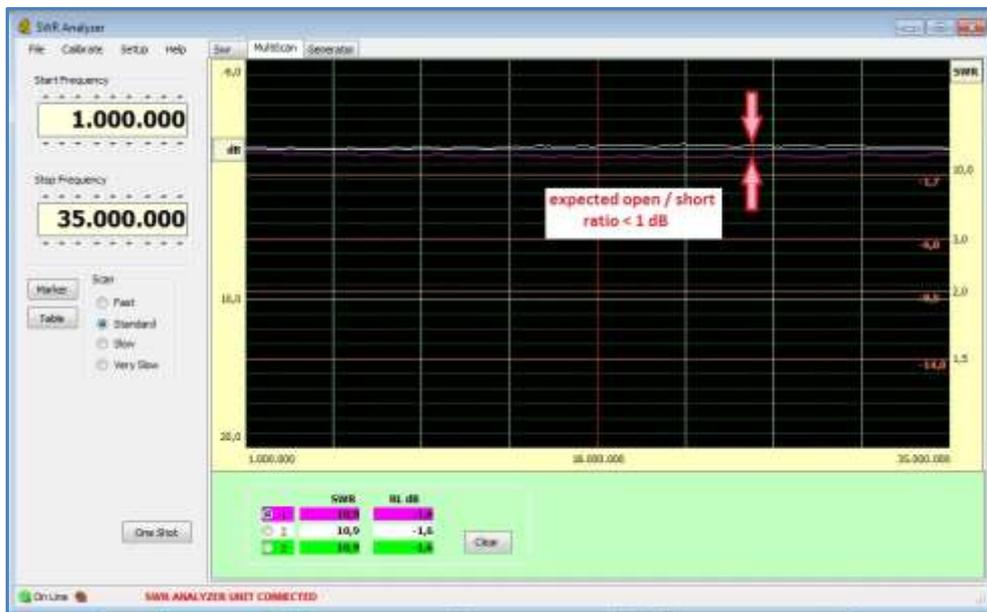
The dB difference of 2 horizontal traces across the whole HF bands, measures the Open/Short ratio.
