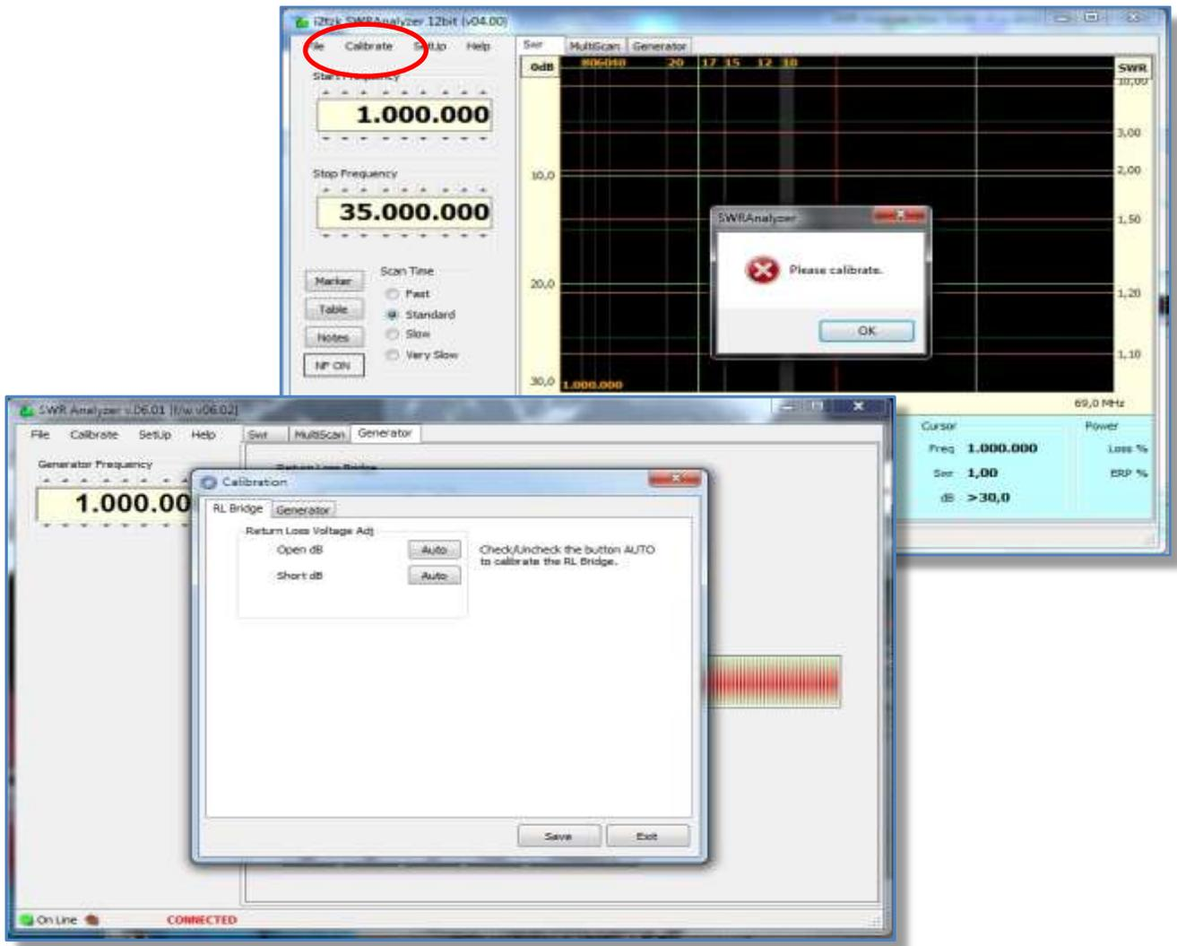
The Calibration window also has a Generator Tab, where the oscillator frequency can be fine-tuned using a calibrated frequency counter connected to the BNC connector. ***This adjustment is not necessary for standard operations.***
