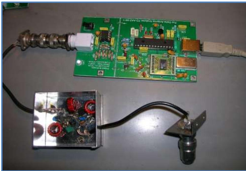
In the figure above the two ports are extended by 50 ohms coax, and the BNC Type dummy load in shown on the right connected to the “L” shaped bracket. It is important to have short and well-soldered terminations to obtain correct results.
