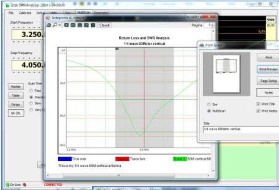
The software enables the user to explore a single HF Band or the full range from 1 to 50MHz on the monitor screen as shown below, or a printed out on paper or save as a PDF or image file (shown on the left) with a title and notes of the investigation for a record to refer to at a later date.
