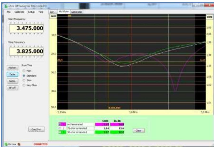
Figure on the left shows three channels being used to compares a pass-band filter response.
