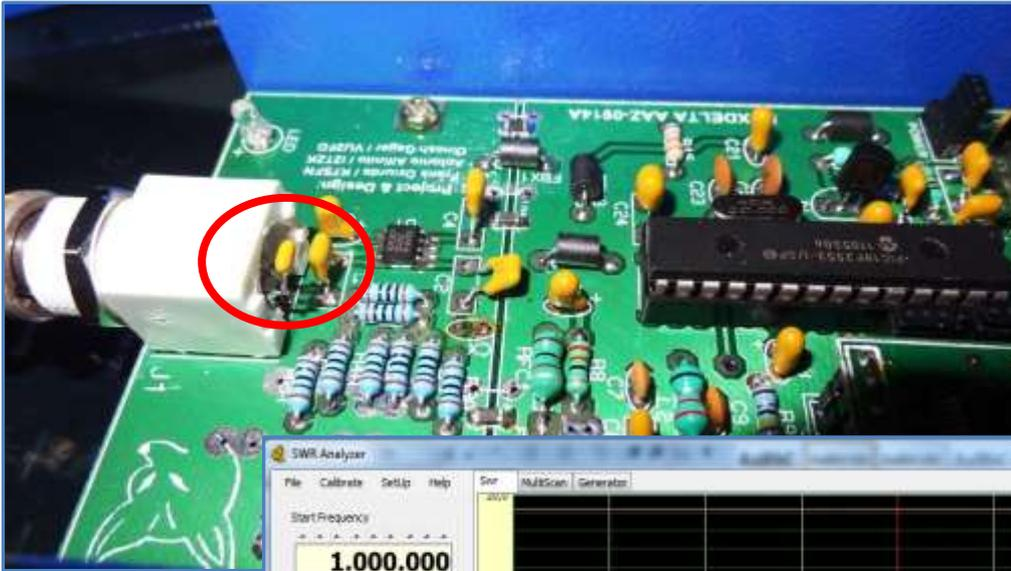
The 50ohm terminator line has been flattened showing a slight variation over the whole HF spectrum; 40.5dB 2 dB @1MHz and 38.5dB @35MHz
