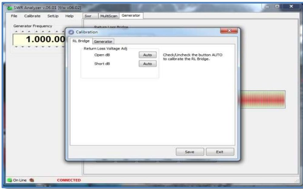
The simple calibration process requires just **2 steps**: Calibration **Open** and **Short** circuit.
