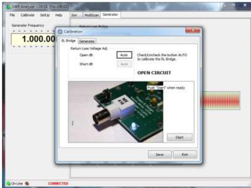
The screen will show the frequency incrementing in 1 MHz steps from 1.0 to 50 MHz.
