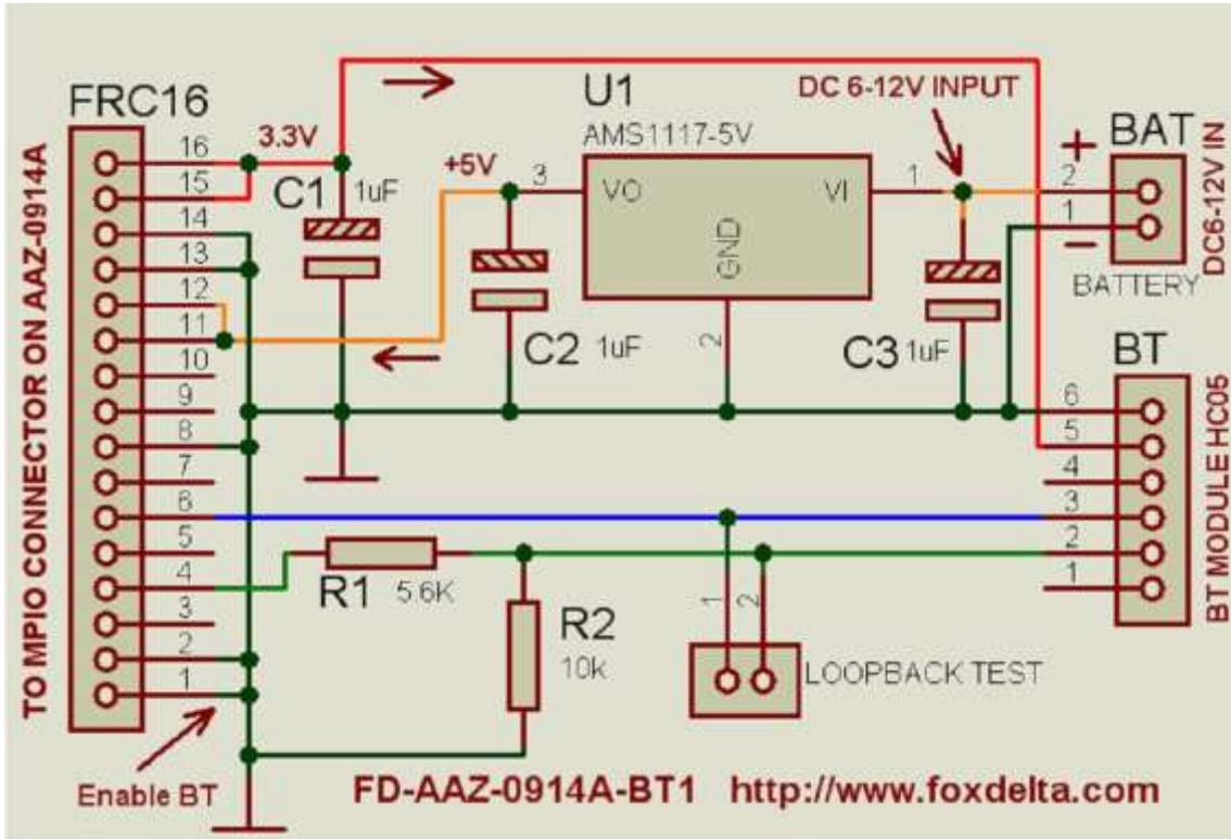
The Bluetooth Module can be powered from AAZ-0914A and it is automatically recognized by the firmware that disables the USB port and activates the Bluetooth communication channel.
