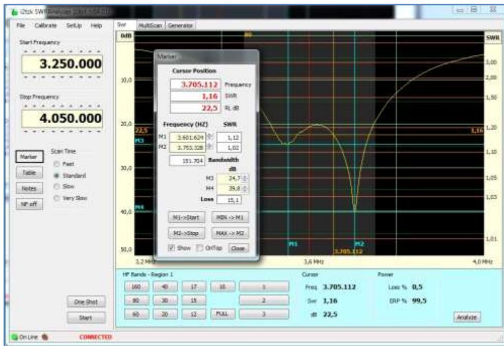
The four markers lines can be moved to specific places on the graph by using the mouse control buttons and keyboard.
