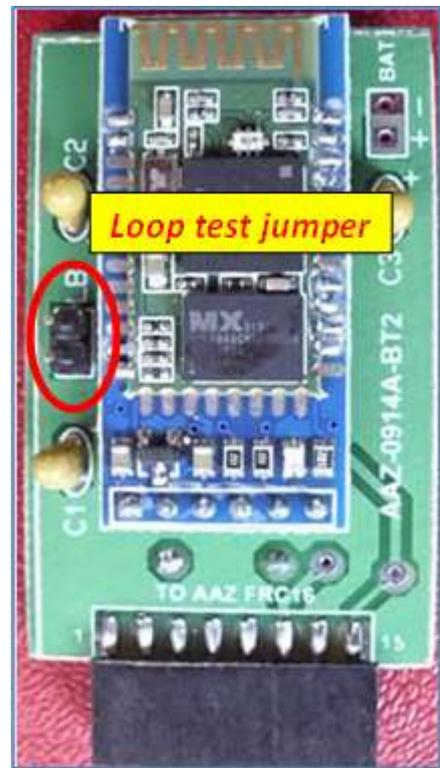
2. Connect and *pair* the BT Adapter to your PC/Smartphone using the 4-digit code specific for the BT module version. The most common code is 1234 for pairing code and HC-05 or HC-06 for ID modules. However, refer to datasheet of the module that is used
