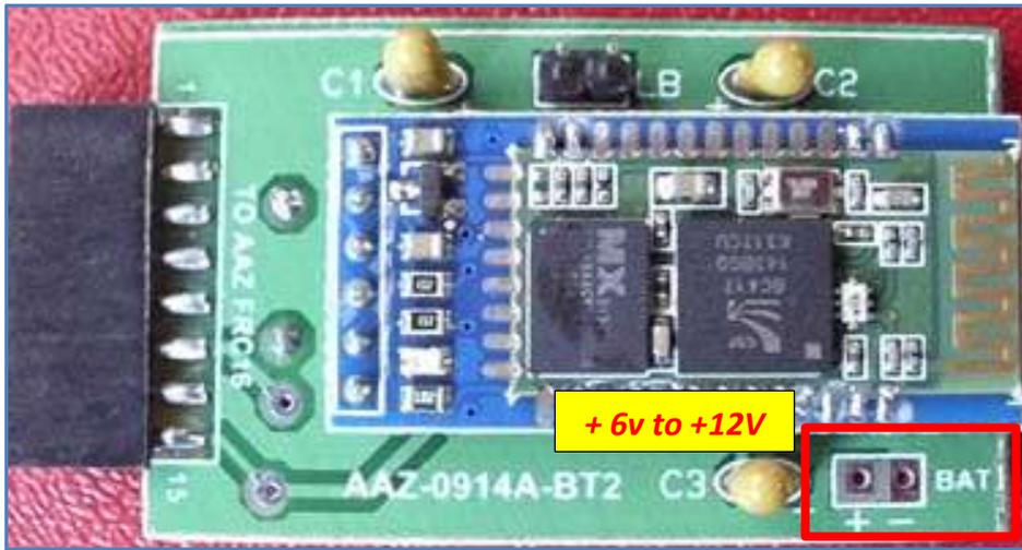
Do not forget to proper positioning the SWRA AAZ-0914A **"POWER" jumper** (refer to the "AAZ-0914A Tech info document" for details).
