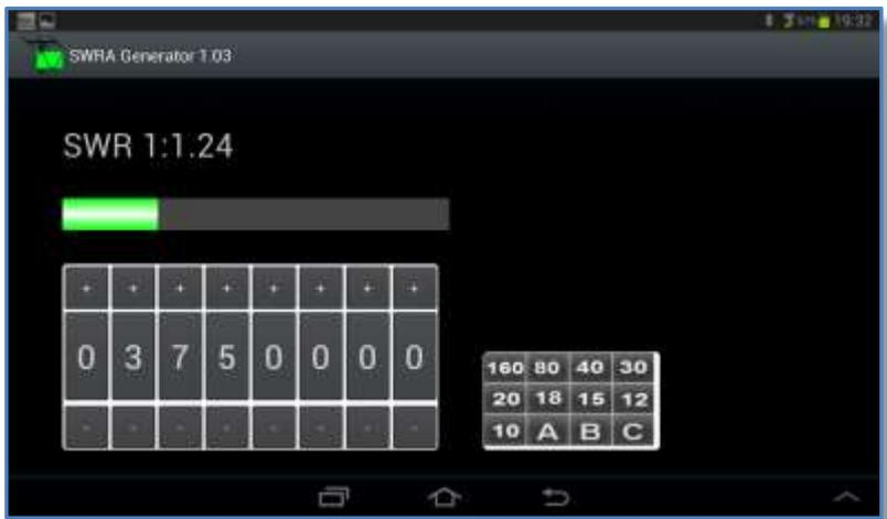
Use the thumb button switches above each digit to select the output frequency
