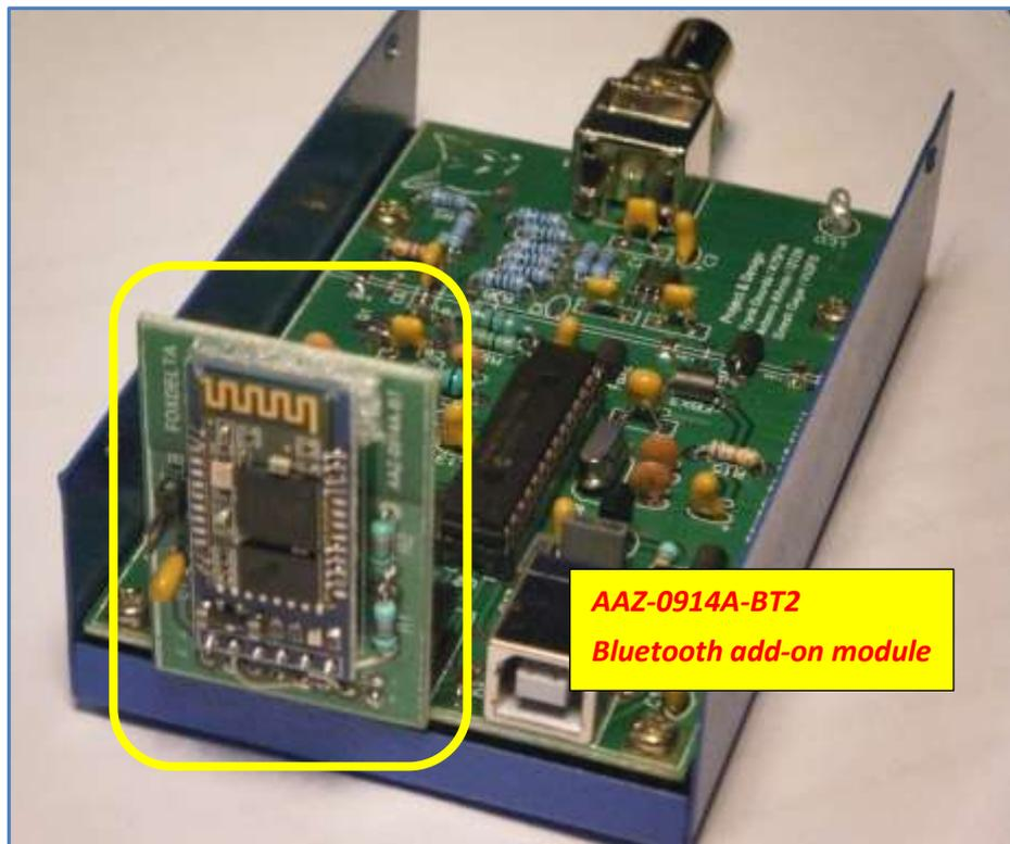
The Bluetooth Module can be powered from AAZ-0914A or from an external power supply and ***it is automatically recognized by the SWRA firmware v6.02 that disables the USB port and activates the Bluetooth*** communication channel.
