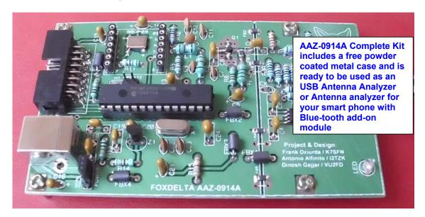
USB Connector Connect to your PC: Supply 5V to AAZ-0914A and establish communication with your PC
