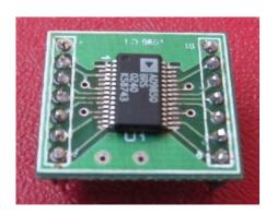
DDS: AD9850 or 9851 will be supplied with kits. (Pre-Soldered and fully tested)
