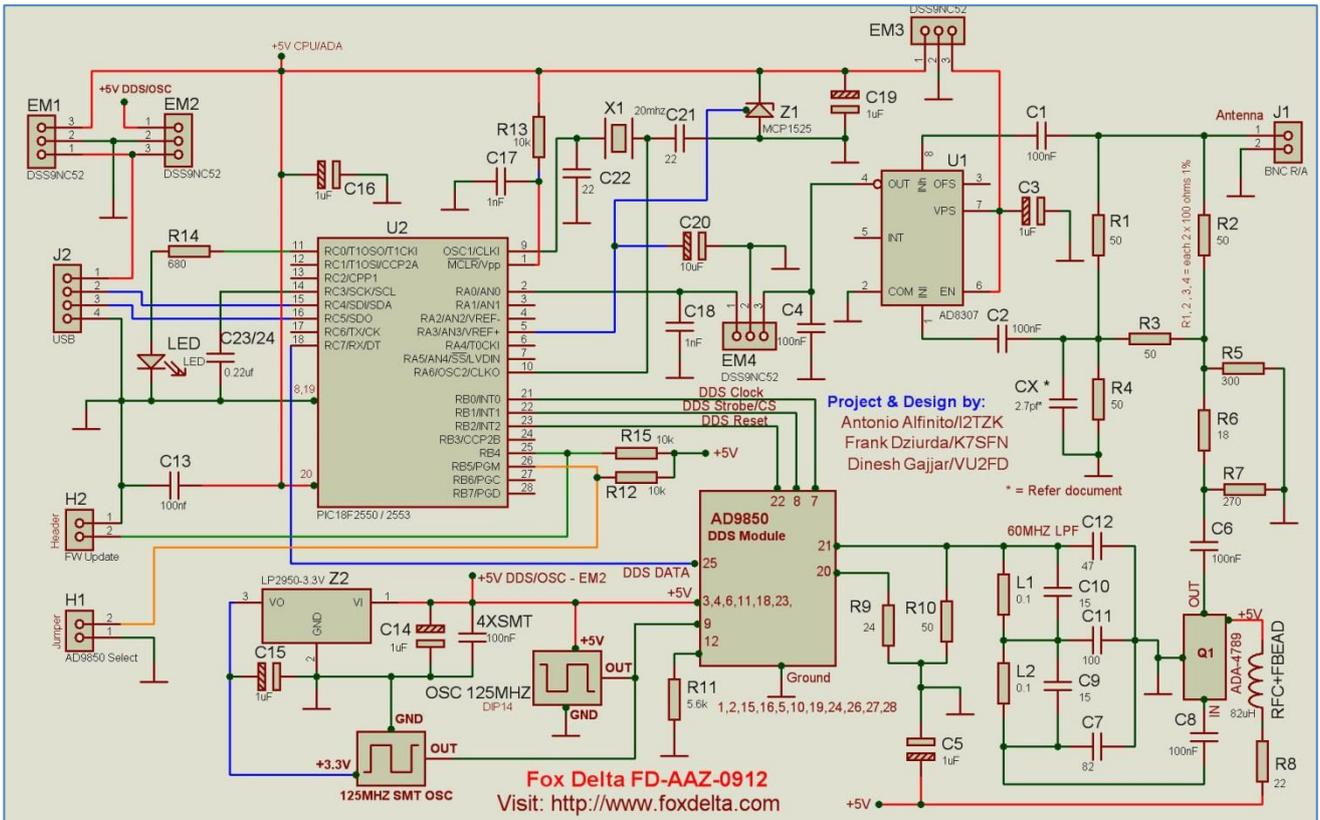
The circuit diagram (FD-AAZ-0912) of the SWR-Analyzer
