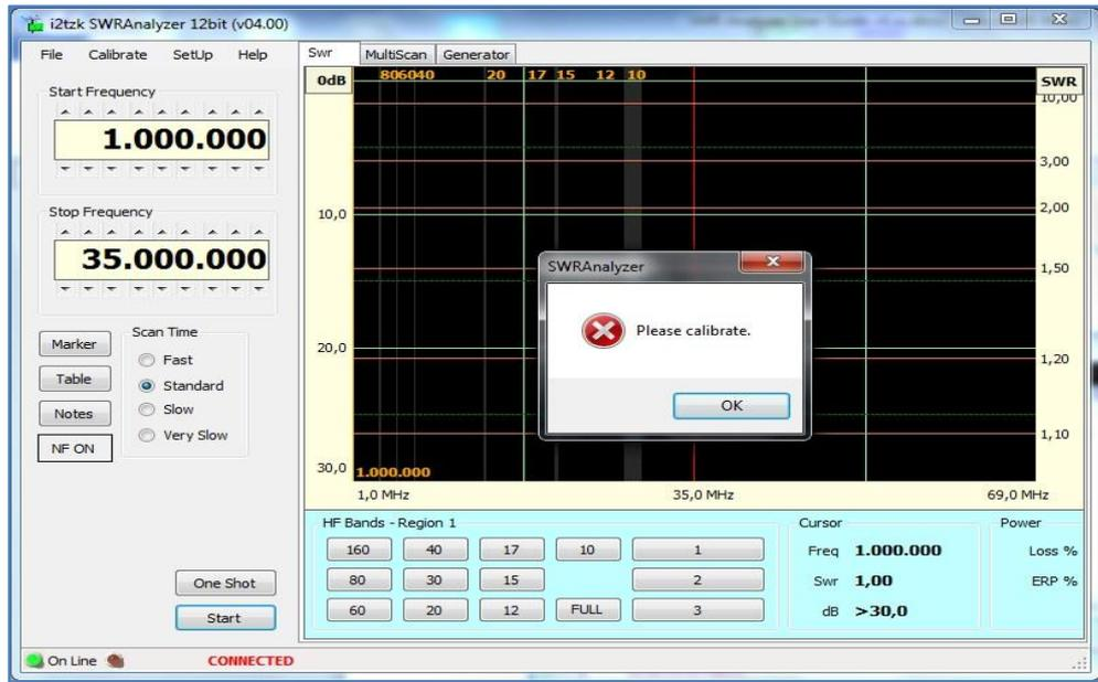
The bridge calibration requires two simple steps: a calibration of the BNC connector with an Open and Short circuit. (A paper clip cut in half is convenient way to create the short circuit)
