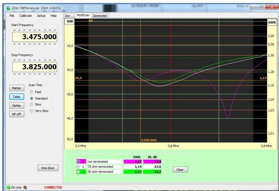
Figure on the left shows three channels being used to compares a pass-band filter response .
