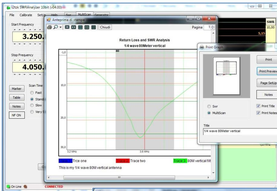
The software enables the user to explore a single HF Band or the full range from 1 to 35MHz on the monitor screen as shown below, or a printed out on paper or save as a PDF or image file (shown on the left) with a title and notes of the investigation for a record to refer to at a later date.
