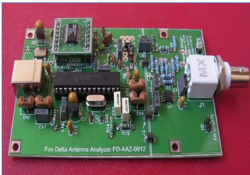
Generally speaking, the higher the DC voltage output, the worst the impedance mismatch is.
