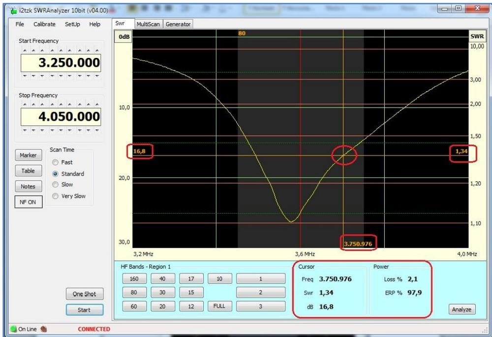
BY moving the mouse over the graphic, two lines (vertical and horizontal) will appear that follow the graphs curve and will continually display the measured values at any position the mouse stops at.
