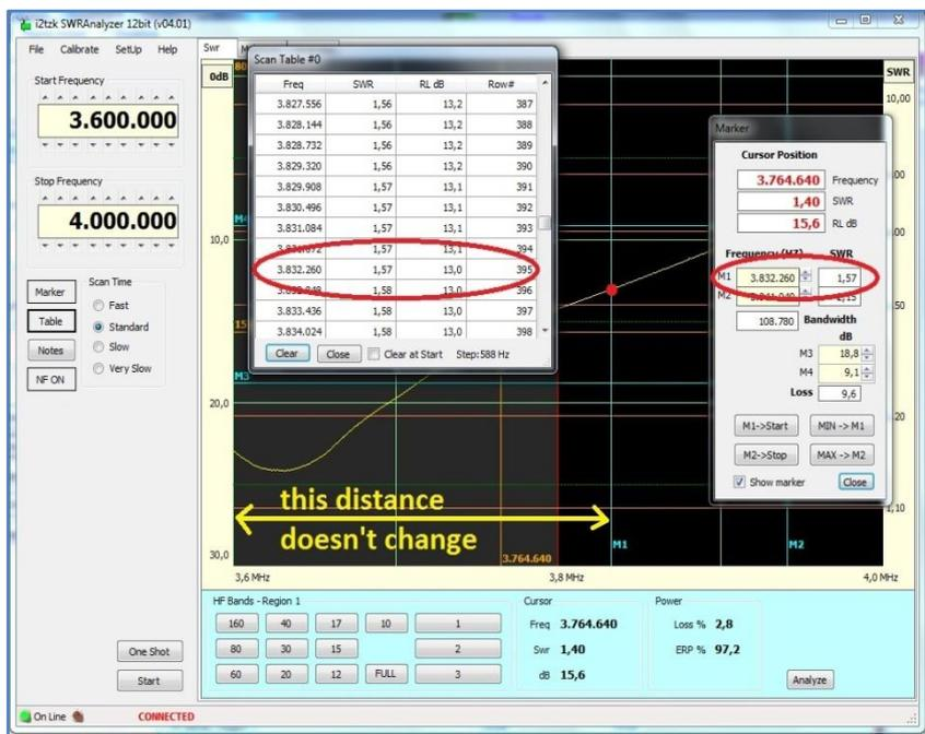
It can be seen that the values and the Scan Table & Marker windows reflect the measured values associated at the frequency, where the M1 marker intersects the graph, i.e. M1 maker is in the same position on the screen in both figures.
