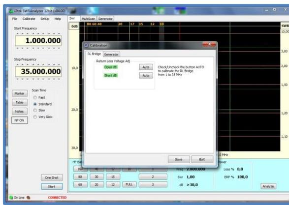
Finally, **[Save]** the calibration data and restart the program. The Program will remember the calibration details and will use this every time you connect the Analyzer to the PS's USB port
