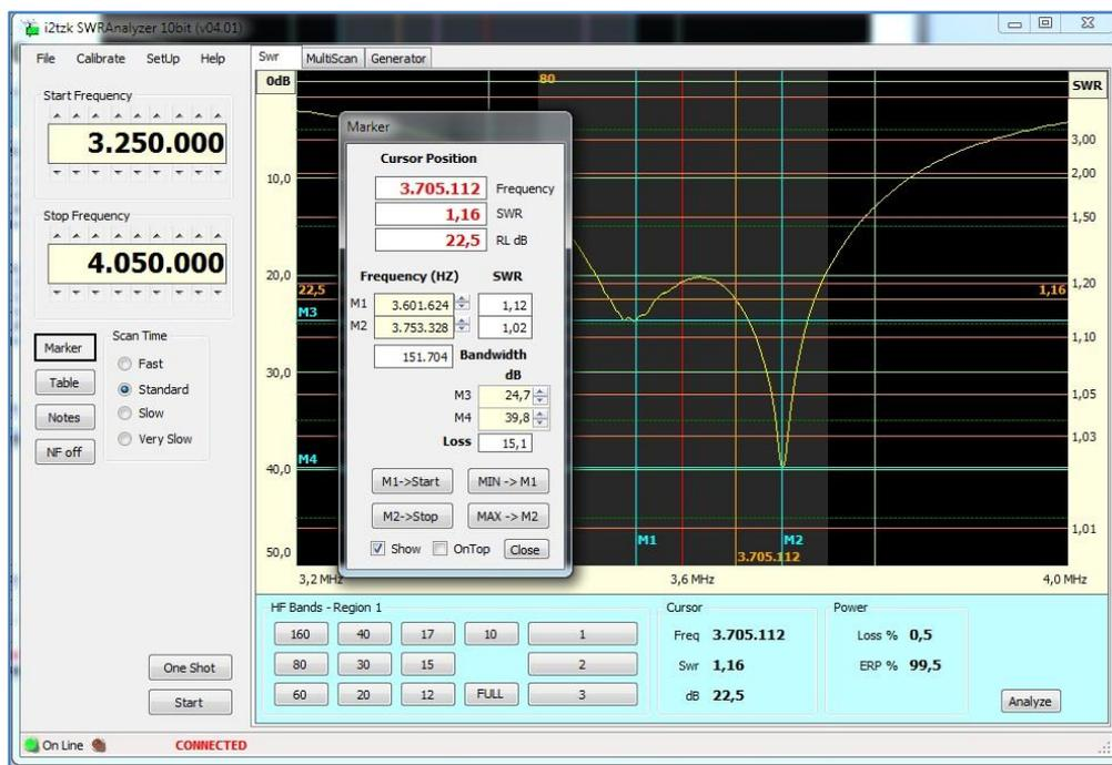
The four markers lines can be moved to specific places on the graph by using the mouse control buttons and keyboard.
