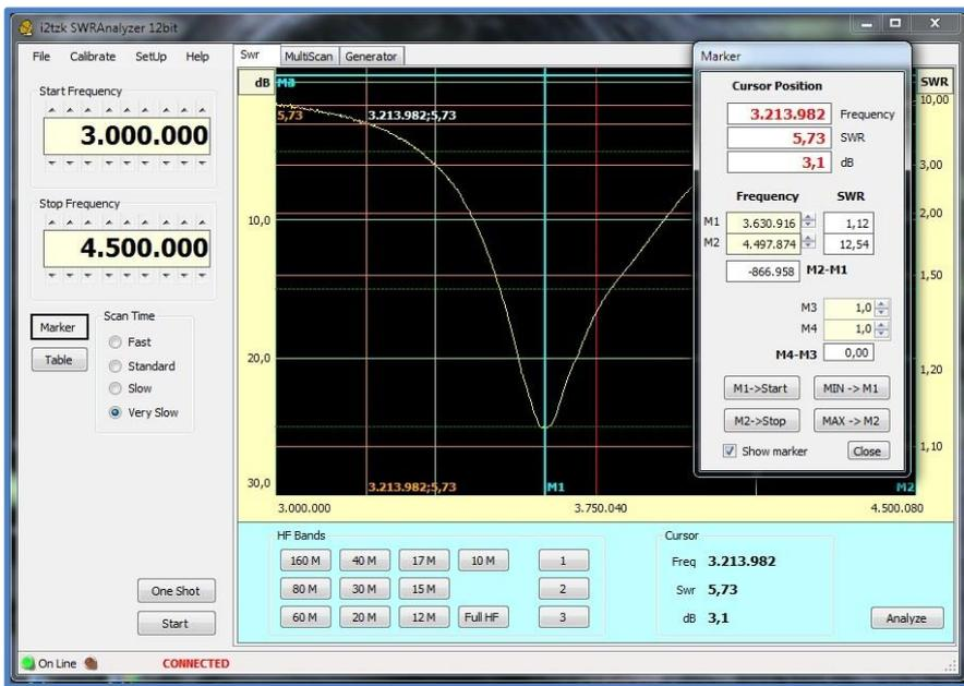
When filter has been tuned, select the [SWR] tab and select the band the filter works in, and click on [One Shot] to view a plot of the filters return loss.
