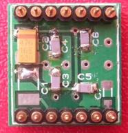
Kit is supplied without AD9851. A set of: Carrier PCB, male/Female headers, 4 X SMT 0.1uf 1206 capacitors and 1 X 22uF/15V Tantalum capacitor are included. You will buy AD9851 and solder it on carrier board and solder SMT capacitors.
