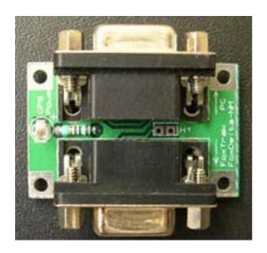
This null modem is a simple 2 x Female D9 PCB which shifts pin 2/3 at one end to 3/2 at the other end.
