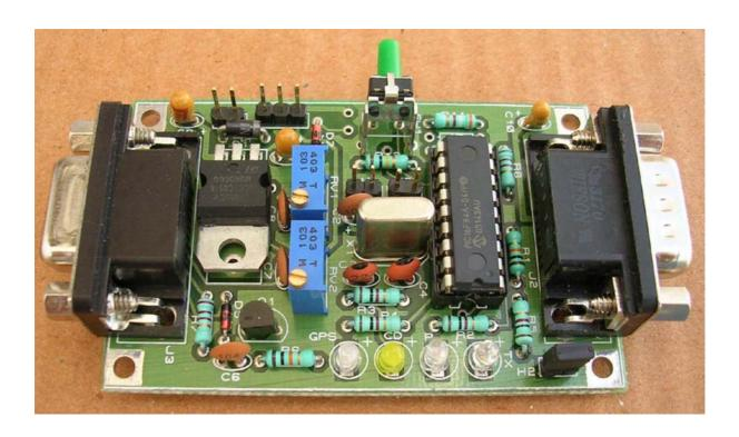
FoxTrak is designed on a Double Sided PTH Board Measuring 7 x 4.5cm
