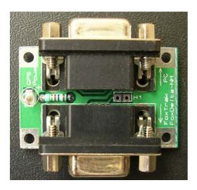
A special null-modem board is designed to use with FoxTrak to configure the PIC parameters. "Null-modem" uses 2 x D9F connectors at both ends and provides reversal of pin 2 & 3 between two sockets.
