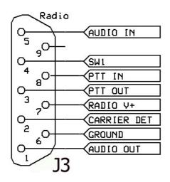
Audio in = Receive Audio from Radio SW1= Instant TX Switch PTT IN = Input of PTT from Radio PTT-OUT = PTT out from Tracker Radio +V = 9 to 15V DC Input Carrier Det. = Squelch from Radio Ground = Radio/Tracker Ground Audio Out: Tracker audio out to Radio MIC
