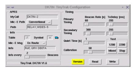
Running any of the 3 config program works well, "Version" should display the version string of the connected FoxTrak as "DK7IN V.1.6".
