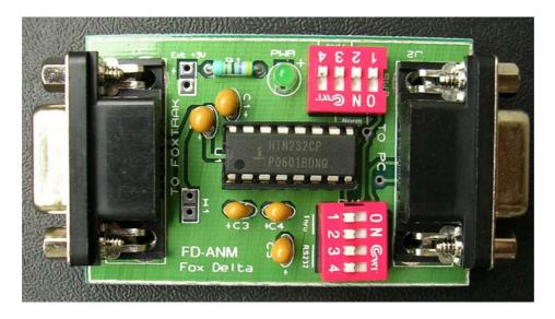
By adding a MAX232 chip & associated components, you may convert passive null-modem adaptor into Active null-modem interface provides true RS232 levels to your PC.
