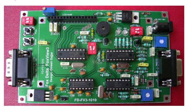
Note: Power may be supplied at J3 or thru the Radio Connector J2 (#7)
