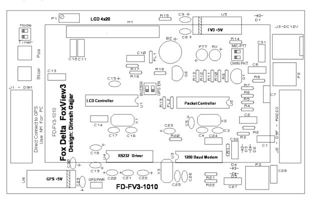
FV3: Rev 1010 uses D9F for Radio and D9M for GPS/PC connection.
