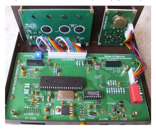
GCPUx is an expandable CPU and Graphic LCD project which has provision to "add" a "project" board to create a full function amateur radio station accessory.
