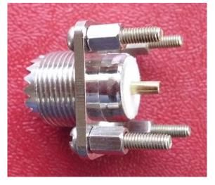
SO239 uses 6mm spacers: Ready for installation
