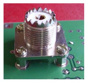
SO239 connectors are suspended by 6MM long brass hex nuts and mounted directly on PCB
