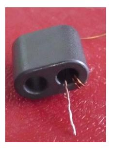
Complete this winding till wire is finished. Tin the other end of wire and proceed for second winding
