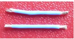
Complete installation of core on PCB and add two 2.5CM links:
