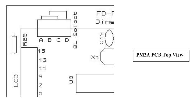
This is basically nothing but reversing DC supply to back light of the LCD (Pins 15 & 16). If you do not know which type of display is supplied to you, just install shorting pins at:
