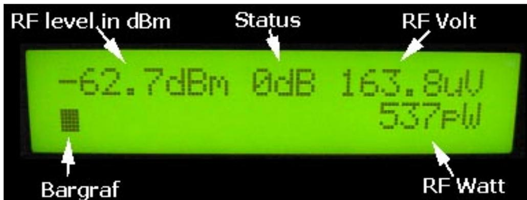
If no attenuator is used, the dBm readout goes from -63 (noise floor) to +30 dBm (1W)
