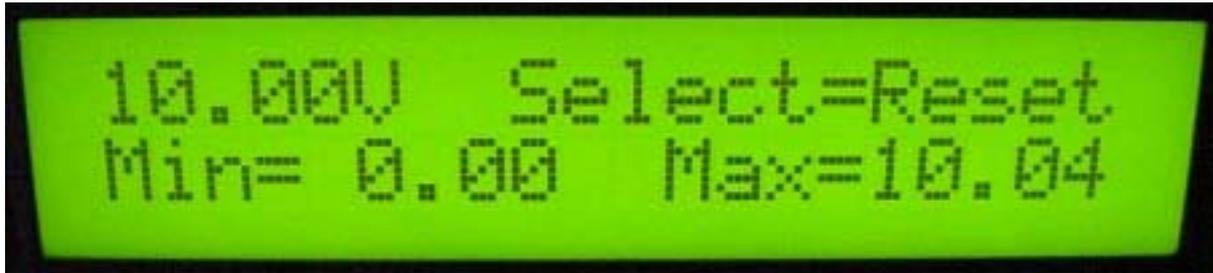
The DC voltmeter can measure from 0 to 20 volt only positive, with a resolution of 20mV. Nothing is burned if input is reversed, it just cannot measure!
