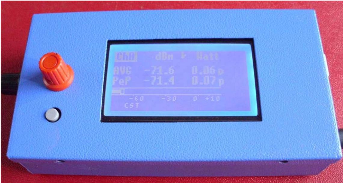
PM4: Graphic LCD/CPU loaded with PM4 Firmware
