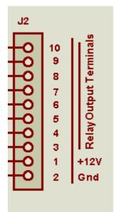
Screw-in terminals are available on board for external connections of relay or other control circuits. Outputs are "OC".
