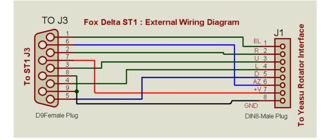
D9M right angle connector is supplied for ST1 to Interface with Yaesu Rotor Controller.
