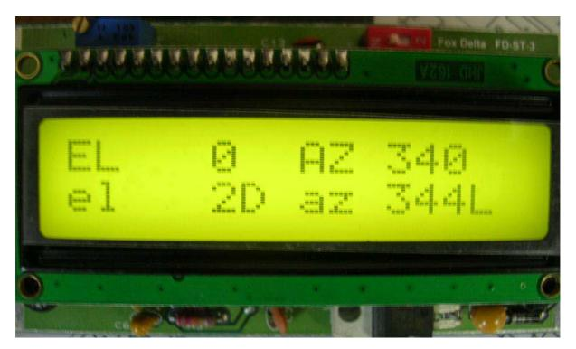
Top line indicates where antenna must, decided by Satellite Tracking Software running on your PC. Second line displays actual position of your antenna.
